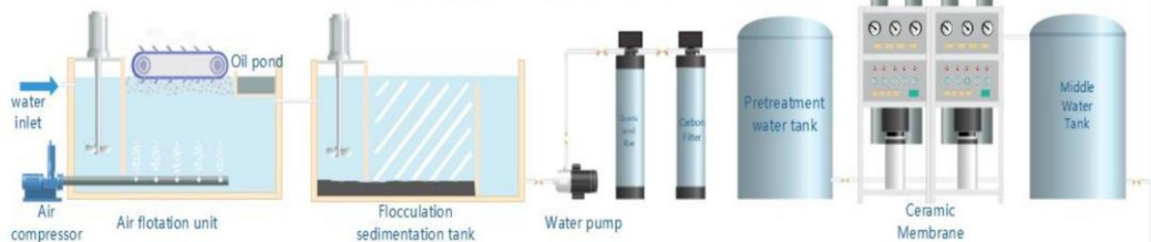
Oily Sewage Treatment Process Flow Chart
